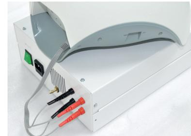
2. Connect the lead wire from output socket of Winstim to input socket of Digital Vacuum at back Side. (red to red and black to black).
